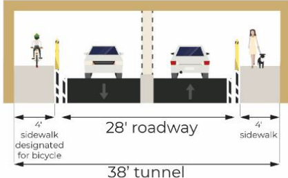
Figure 22: Proposed Viaduct Section - No Change in Width
